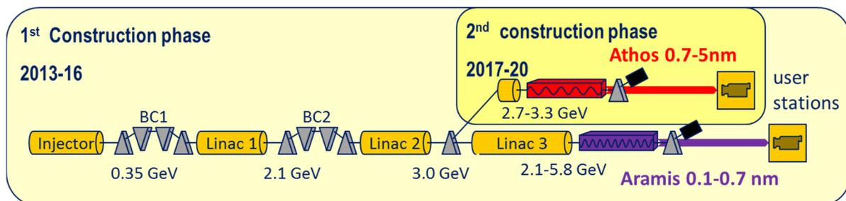
Figure 1: Schematic SwissFEL accelerator layout.
