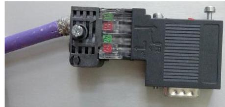
Figure 6: Deteriorated cable in a Profibus connector.
