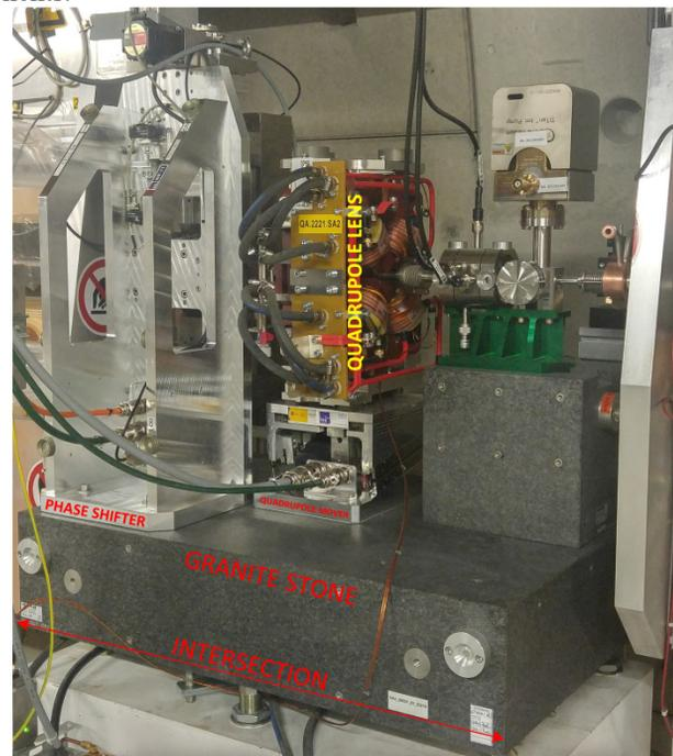
Figure 3: Intersection components installed on the granite stone in the tunnel and connected to the undulator control system.
