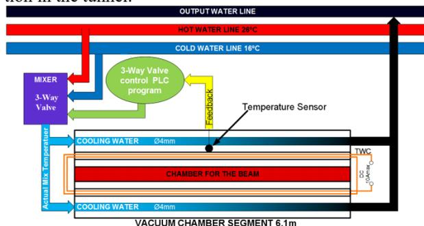
Figure 2: Schematic view of the parallel water connection scheme and the control system of the mixer. Two wire connection system (TWC).
