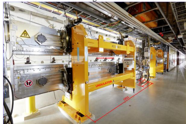
Figure 1: The view of SASE1 cell, equipped with the undulator system components: vacuum chamber, undulator, intersection, UCR and ICR.
