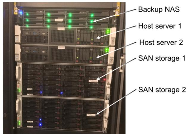
Figure 4: ACS rack with servers, storage and NAS box for backups.
