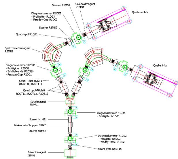
Figure 1: Former LEBT with two ion sources.
