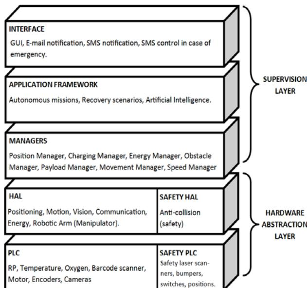
Figure 5: Control system design in layers.
