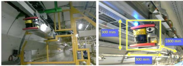
Figure 3: TIM in the LHC tunnel passing sector doors (left) and the dimensions of one wagon (right).
