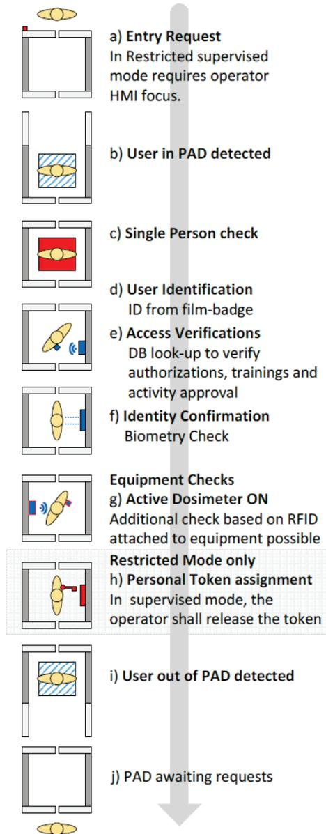
Figure 1: SPS PAD Entry Cycle.
