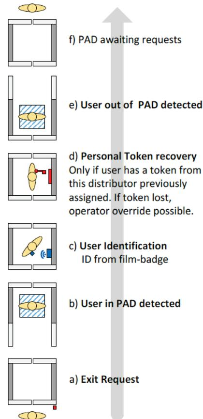
Figure 2: SPS PAD Exit Cycle.
