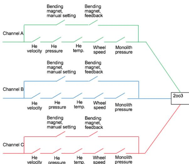
Figure 3: Logic for 2003 voting of the channels.
