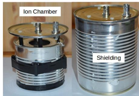
Figure 3: Ion chamber made from cylindrical cans. The outer can provides a shielding against high frequency signals, for further details see text.
