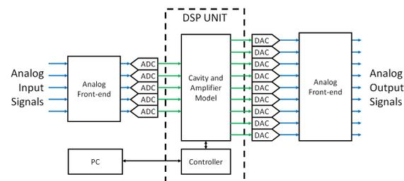
Figure 2: The simplified block diagram of the Cavity Simulator.
