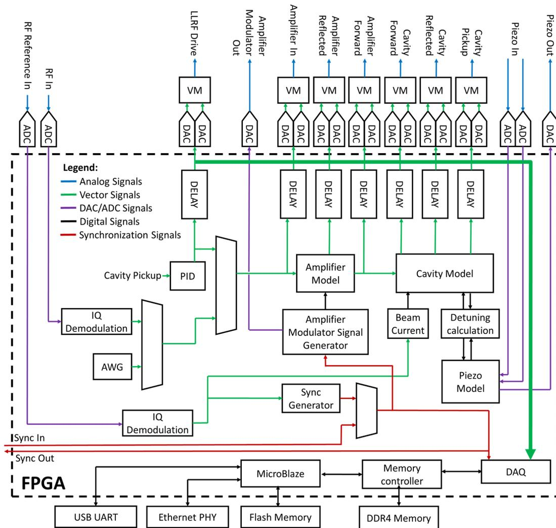
Figure 6: The block diagram of the Cavity Simulator firmware.
