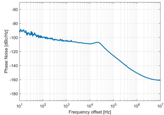
Figure 5: The expected phase noise spectrum of the signal generated by the Reference Generation Module.
