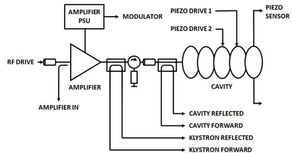
Figure 1: The block diagram of the system simulated by the Cavity Simulator
