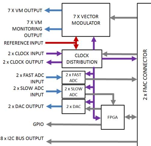
Figure 4: The Block Diagram of the Data Converters Module
