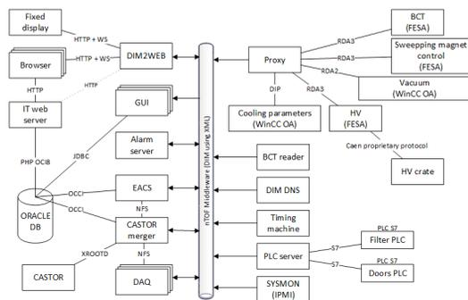
Figure 4: nTOF DAQ software architecture.
