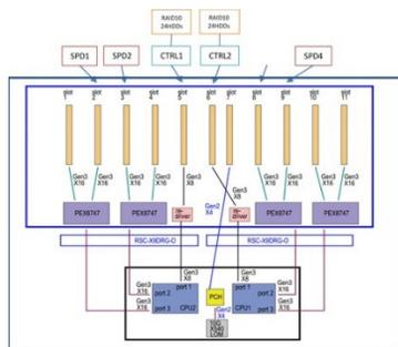
Figure 2: DAQ unit hardware architecture.
