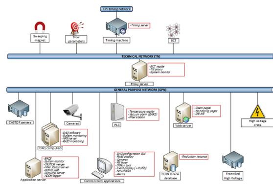
Figure 1: n\_TOF DAQ hardware architecture.
