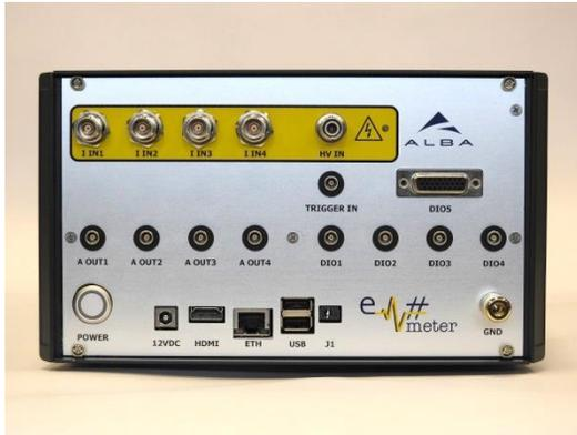
Figure 4: Rear panel of Em#\_HV.
