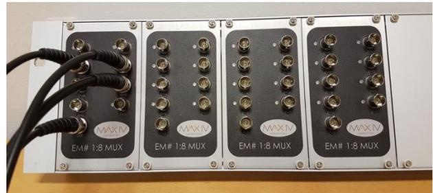
Figure 7: An 8 channel multiplexer. Up to 4 multiplexers can be interfaced by the same electrometer.
