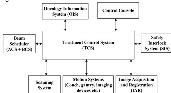
Figure 1: Overview of the treatment control system.
