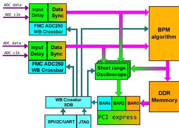
Figure 3: Example block realisation of the DAQ with data processing path enabled.
