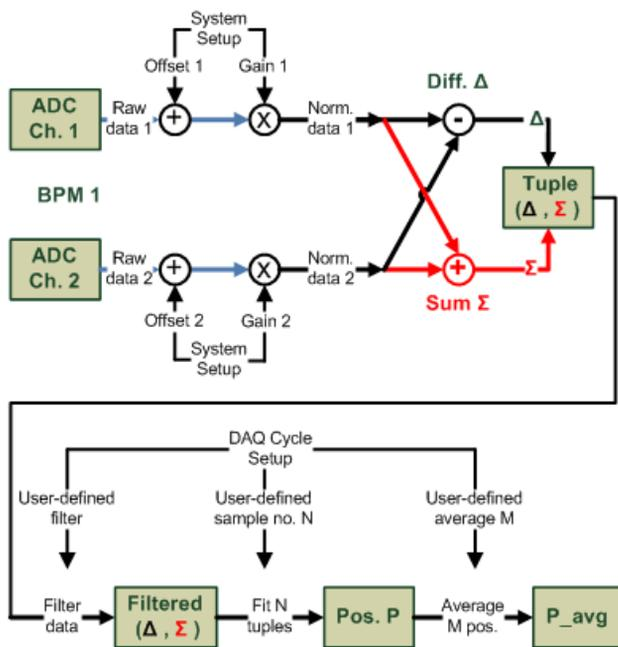
Figure 5: BPM signal flow during the digital processing in the FPGA.
