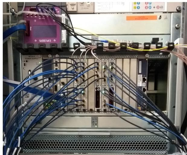
Figure 2: BPM DAQ system in  $\mu$ TCA form factor.
