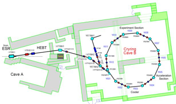
Figure 1: Scheme of CRYRING installation in Cave B.
