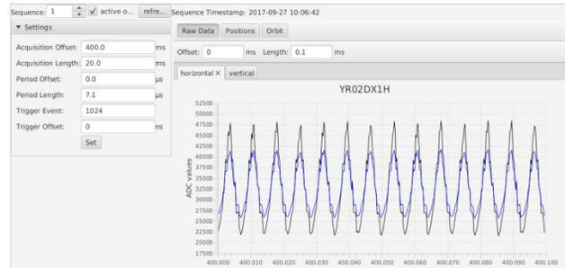
Figure 6: Real raw data BPM signal of the new DAQ system with 300 keV/u  $H_2^+$  beam.
