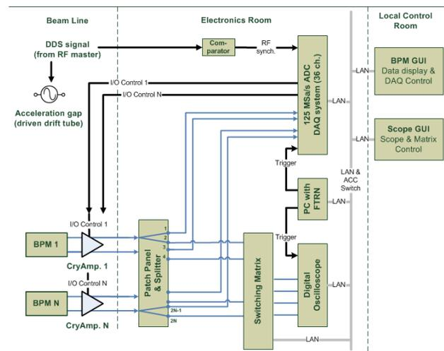
Figure 4: Schematic of the BPM signal chain and acquisition system.
