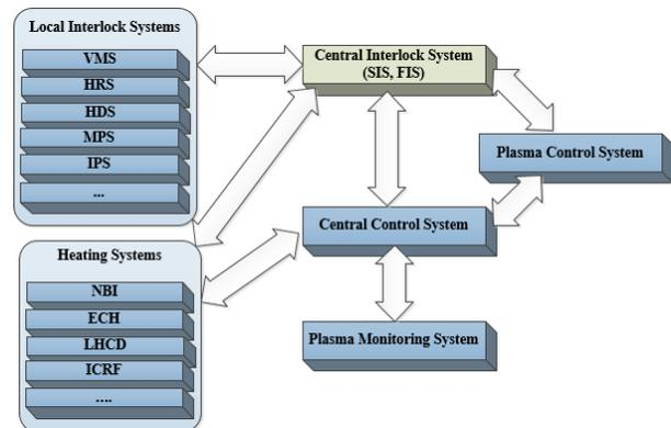
Figure 1: Interlock related system interface.
