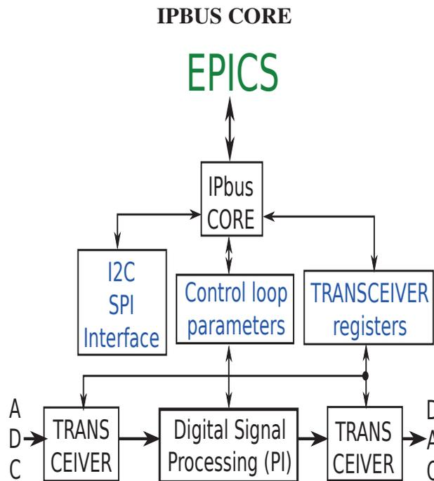
Figure 2: Block diagram of the firmware implemented.
