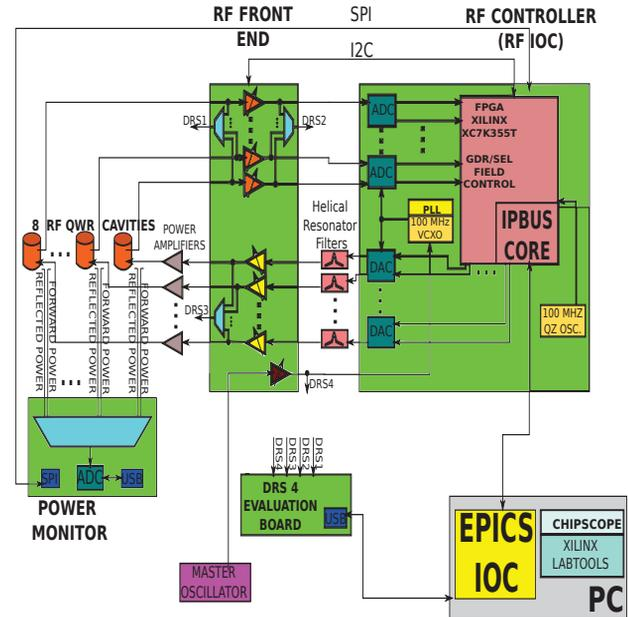
Figure 1: Block diagram of the LLRF system
