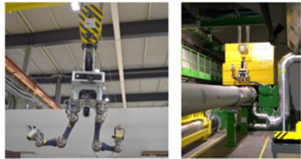
Figure 8: CERNbot core in dual-arms configuration integrated on a crane for accessing complicated areas.
