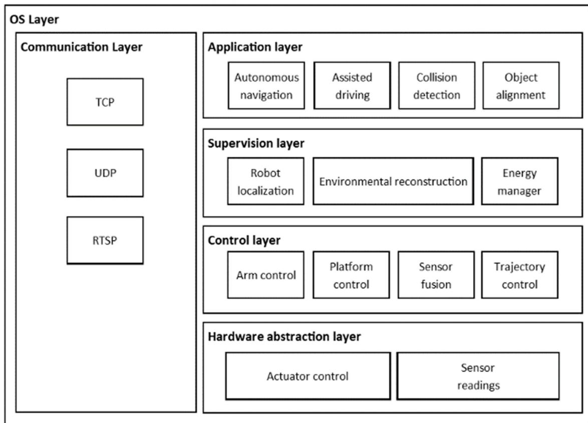
Figure 3: CERNbot control system architecture.
