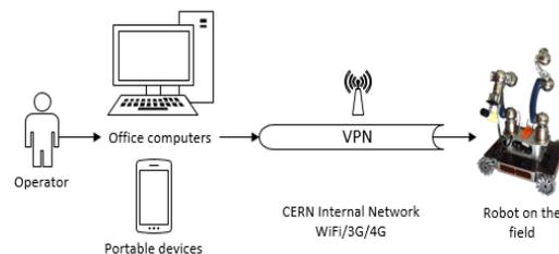
Figure 5: CERNbot basic communication scheme.
