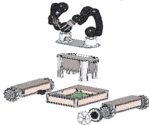
Figure 2: Different CERNbot hardware components.
