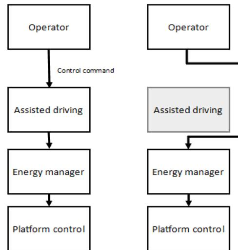
Figure 4: Automatic IPC redirection after suspension of assisted driving module.
