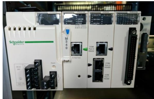
Figure 5: Example of Schneider Electric M340 PLC.
