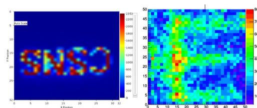
Figure 9: Left: the image of CSNS mask under X ray, right: the image of E mask under  $^{252}\text{Cf}$  neutron source
