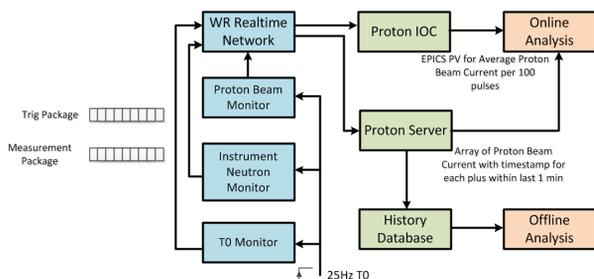
Figure 5: Proton current measure and service.
