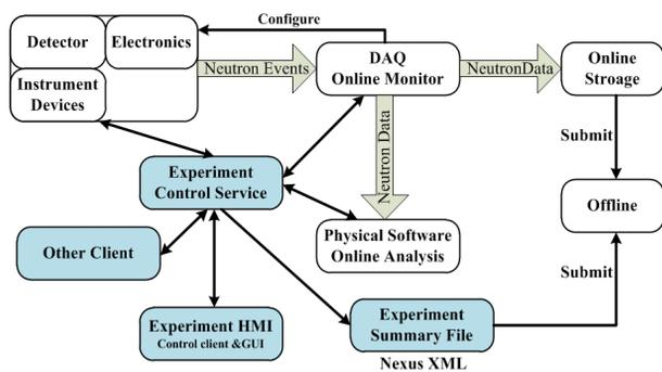
Figure 7: The data flow of CSNS neutron instrument
