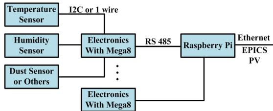
Figure 3: the low cost environment monitor
