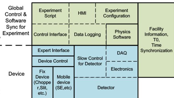
Figure 2: The Structure of CSNS Instrument.
