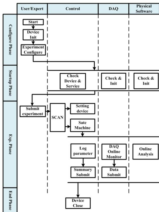
Figure 6: The flow of neutron experiment in CSNS.
