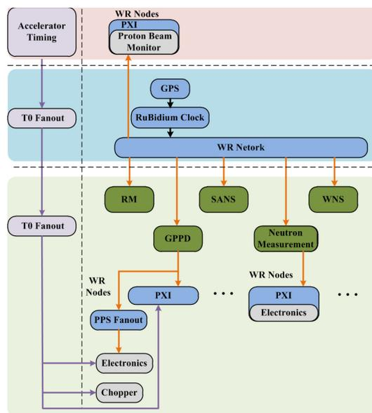
Figure 4: Time synchronization and realtime measurement system..
