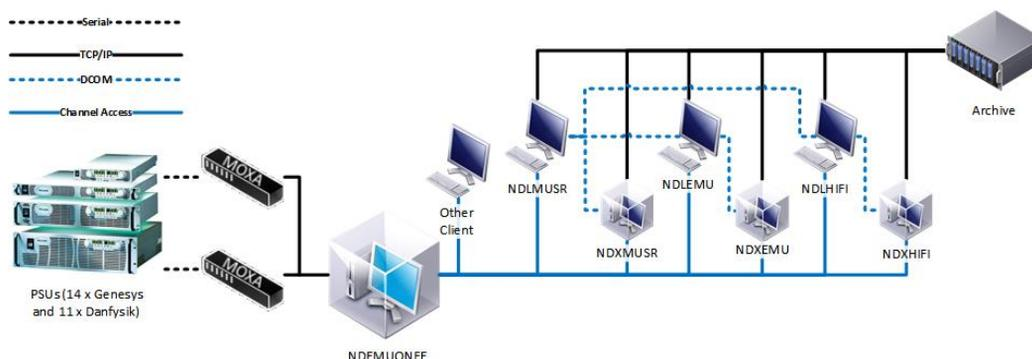
Figure 1: Hardware and computer overview of the muon front end system.
