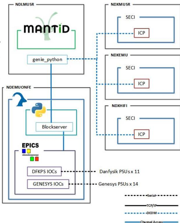
Figure 2: Software overview of the muon front end system.
