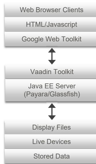
Figure 2: System diagram and tools.
