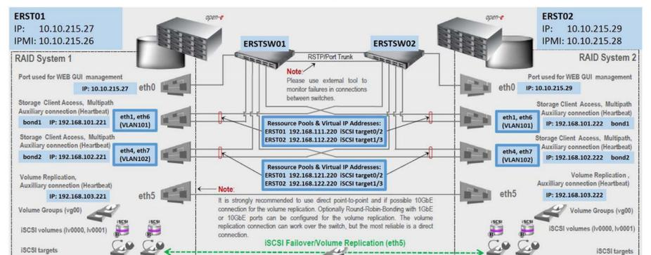
Fig. 4: Concept for the ACS Server Storage with 10GbE network iSCSI.
