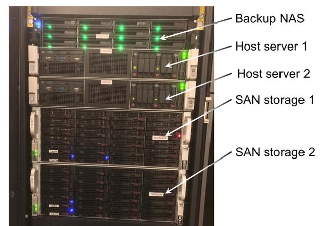
Fig. 3: ACS rack with servers (middle), storage (bottom) and NAS box (top) for backups
