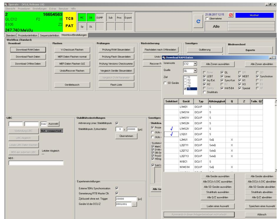
Fig. 2: Improved download GUI with selection window open. The flash GUI looks identical. The download will be checked against checksums in the database and repeated up to 3 times. Checksums can also be verified manually.
