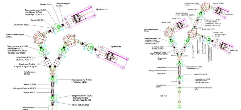
Fig. 1: left: old LEBT with 2 ion sources right: new LEBT with 3 ion sources
