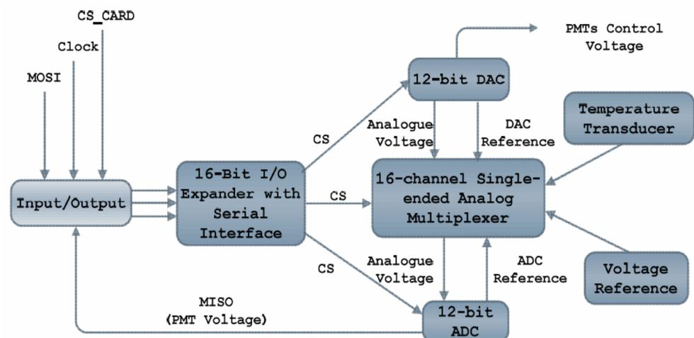
Figure 3 – Block Diagram of the HVRemote-Ctrl Card.
