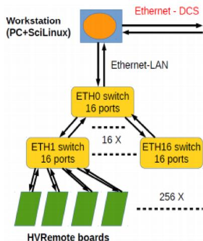
Figure 1 – Architecture of HVRemote Control Tree
