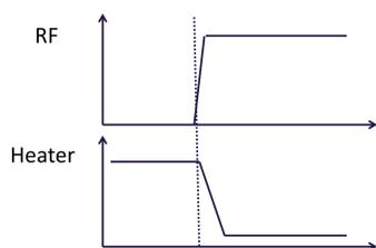
Figure 1: Heater power decreasing while RF power increases and thus dissipates the same amount of heat into the LHe bath. The overall energy balance stays constant.
