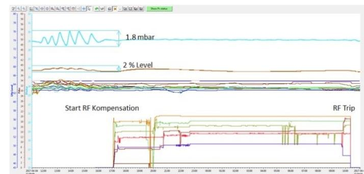
Figure 4: First run with heat load compensation switched on. And first RF trip the next day.
