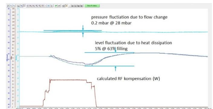
Figure 5: 'Soft quench' of just one cavity can cause major problems in a cryo string.
