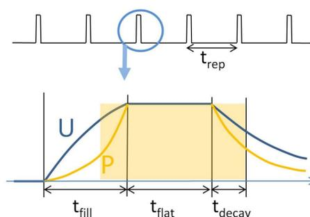
Figure 3: Repetition rate and pulse form.
