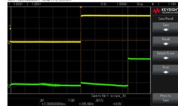
Signal output timing at the BIS2 between other stations (3.38 ms, Average response time : ~ 3.8 ms)
