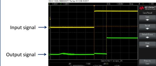
Signal output timing at the BIS2 within the same station (1.40 ms, Average response time : ~ 1.4 ms)
